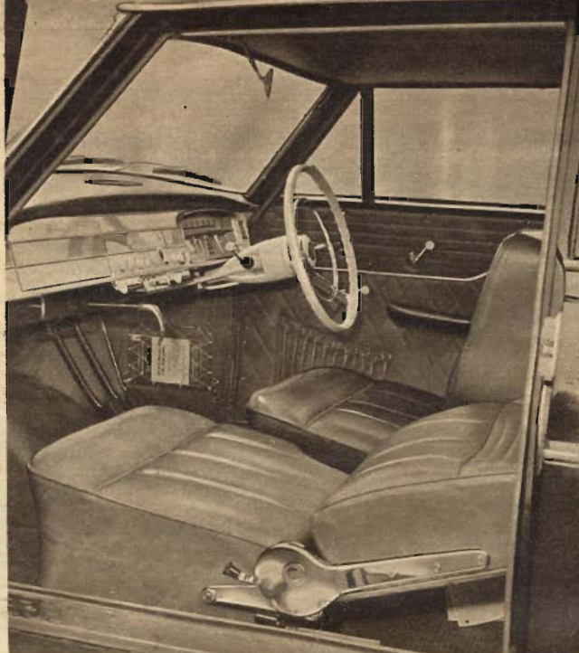
The TS Isabella is fitted with separate front seats by Reutter. Each backrest may be adjusted for rake by a small lever. The backrests will mate with the edge of the rear seat cushion. There is a single armrest for each of up to four occupants
