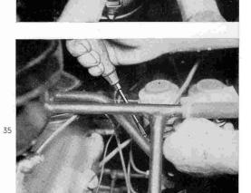
Remove rubber grommet for speedometer drive on body wall and pull out speedometer drive forward. (Screwdriver).
