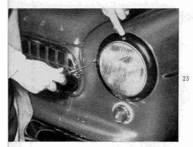
4. Separate lamp carrier by tipping of the tension clip from headlamp, remove headlamp.
